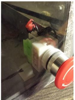
Above are final pictures of the emergency stop button installed. I used a step drill bit to drill the **7/8" through hole** for the button.
